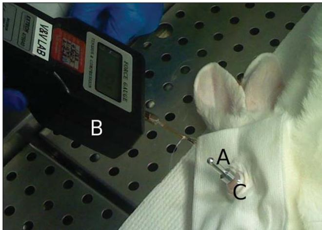
**Figure 2.** Flap adhesion strength measurement. A plano-concave acrylic lens with 10-mm radius of curvature (not visible), attached to a customized aluminum holder (A), was glued to the flap after removal of the epithelium and pulled with a tension meter (B). The peripheral cornea and sclera are visible (C) next to the aluminum holder (A).
